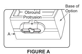
Push the obround protrusion through any obround opening in your desired location on any universal mounting system (UMS) pattern. (FIGURE B)
